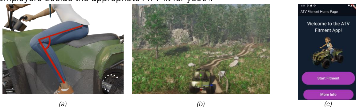
Figure 1. (a) One of the 11 reach evaluation criteria for riding ATV: Upper leg angle, (b) ATV riding simulator screen, (c) Screenshot of ATV fitting App.
